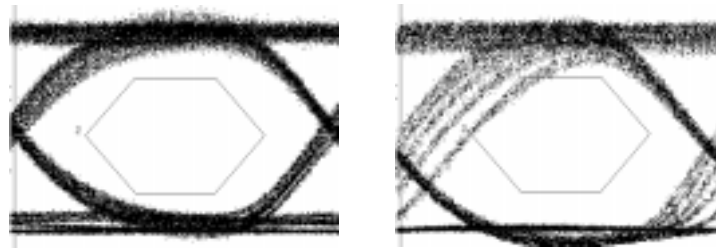
Figure 9. Eye diagram of a single VCSEL: properly biased (left) and biased too far below I_{TH} (right), with resulting jitter. (Fibre Channel K28.5 pattern.)
