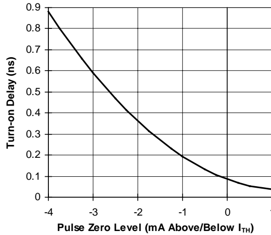
Figure 8. Turn-on delay as a function of distance from I_{TH} .
